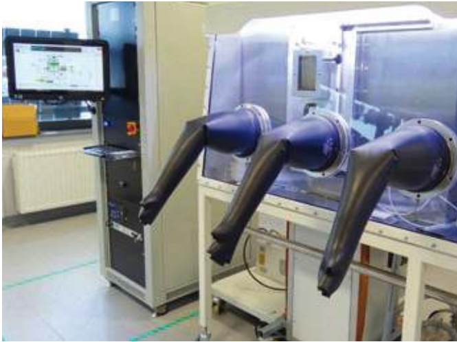
System for deposition of the thin layers with the gloves box
