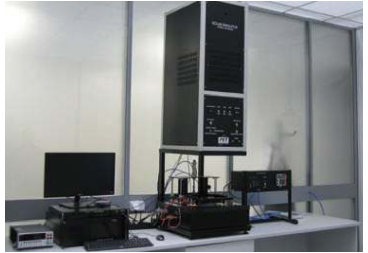
Solar simulator for single PV cell testing
