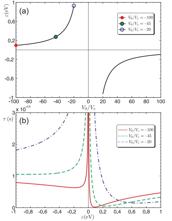
FIG. 1. (Color online) (a) Energy of the resonant states as a function of the impurity potential  $V_0/V_c$ . (b) Momentum relaxation time  $\tau$  as a function of electron energy  $\varepsilon$ , calculated for the impurity concentration  $N_i = 2 \times 10^{14} \text{ m}^{-2}$ , and for the resonant states (and  $V_0/V_c$ ) corresponding to the points marked in (a).
