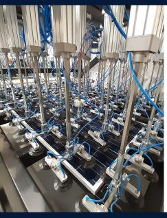
Resistance of the PV module to wind
