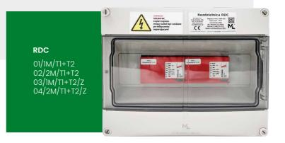
HUN: IP65 switchgear with surge protection DEHN T1+T2 protecting the MPP Tracker of the inverter. In the RDC03/IM/T1+T2/Z and RDC04/2M/T1+T2/Z models, the connections are made by Phoenix Contact spring bar terminal blocks with the option of paralleling inside the housing.
