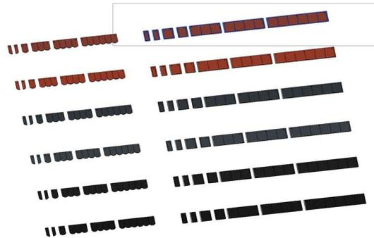
In order to place the tiles in your model, simply select them from Component tab and place on a model or work plane. Horizontal Axis is aligned with rooftile openings and should be placed on battens axis. You can also use simple battens family that is also included in our Project. You can then use array and align tools to populate whole roof.
