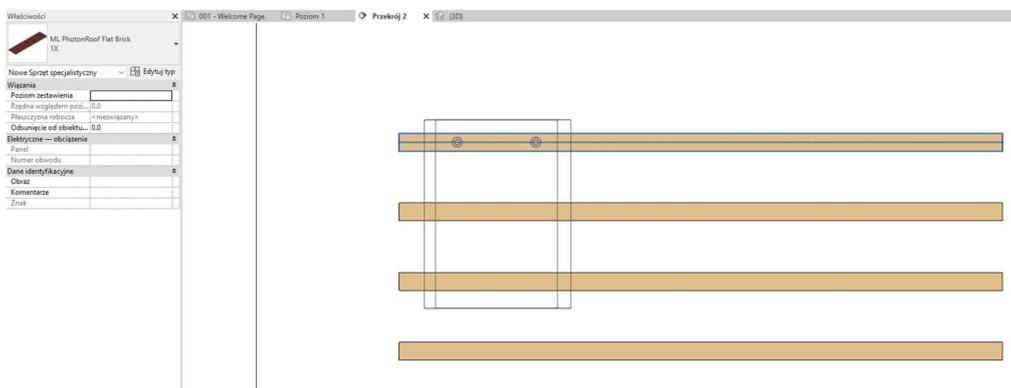
Family types are locked to a standard battens spacing. This assures right angle, so Rooftiles are not colliding in the model. In case you need to use different battens spacing, you can change it – but you have to do it for every tile separately. However changing that is not necessary – the differences are not big enough for rooftiles to collide in the model.
