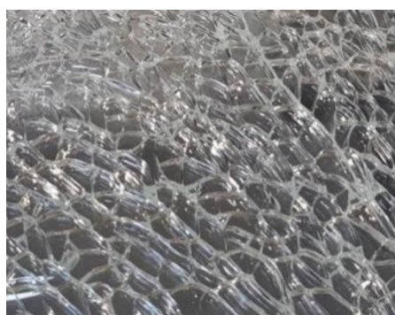
Fig. 16. Fragmentation pattern of tempered glass
