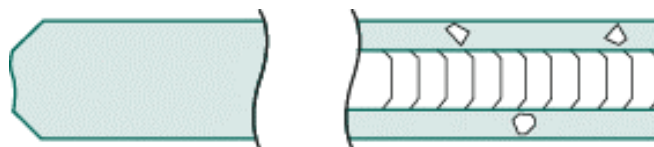
Fig. 7. Arrissed glass edge.
