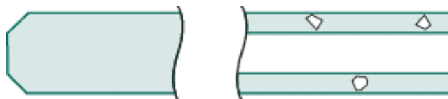
Fig. 8. Ground glass edge.
